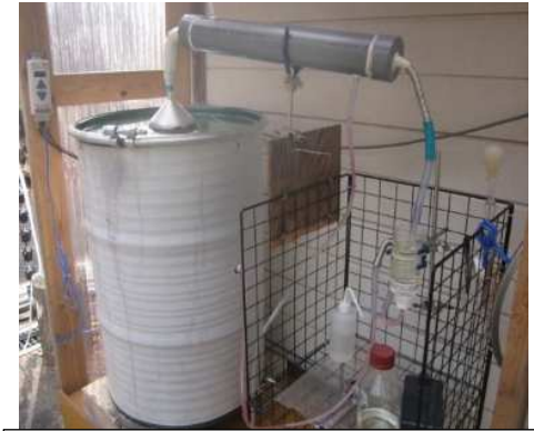
Essential oil extraction machine developed using drums
